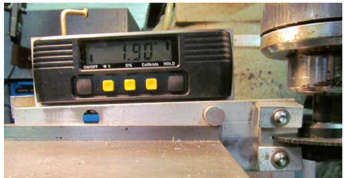
gently approach until contact is made. Zero the left-right feed and advance the table L units to the right. This produces the right side of the slot.
